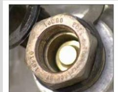
Relief valves in MF cylinders must be replaced within 12 years of the date of manufacture of the cylinder and every 10 years thereafter (the cylinder or valve must be marked). Relief valves must have the proper capacity for the size of the cylinder in which they are installed, and have a start to discharge pressure setting of 375 psig.
