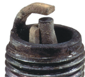
DAMAGED SPARK PLUG
